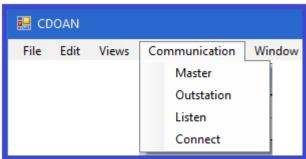
The *Communication* pull-down is used to starts active communication in either master or outstation simulation mode, or listening, and to stop an active communication session.
